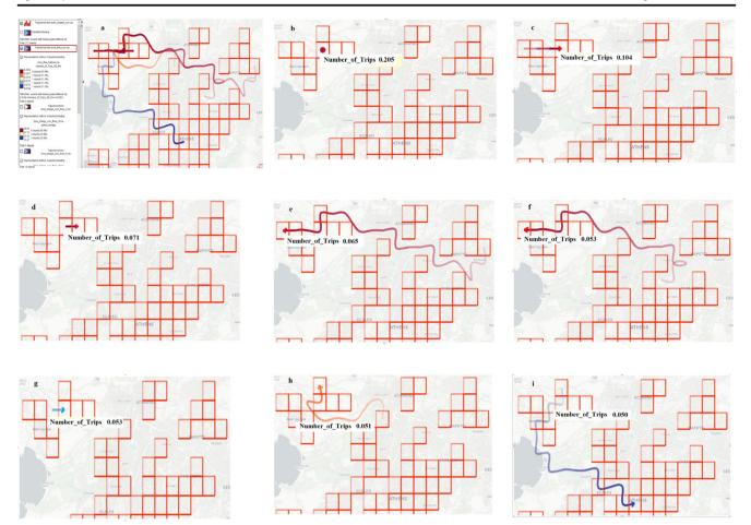
Fig. 10 Major sources of traffic flows in  $Z_{224,189}$  (travel flow layer). Note: the black and red grids are  $Z_{224,189}$  and congestion zones, respectively. The curve describes the typical path Path<sub>od-con</sub> and the attribute window lists the value of  $M_{od-con}$ . **a** displays all the 8 paths and **b**-**i** depict each of these paths
