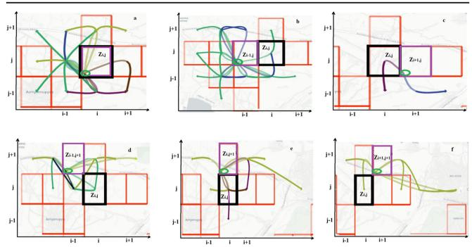
**Fig. 7** Visualization of the road linkage matrix RL in the surrounding area of  $Z_{i,j}$  (road linkage layer). *Note*: the black, purple, and red grids denote the selected zone  $Z_{i,j}$  (i.e.  $Z_{224,189}$ ), the zone where the connections start, and the congestion zones, respectively. Each curve describes the connection among 3 zones, starting from the green circle in the 1st
