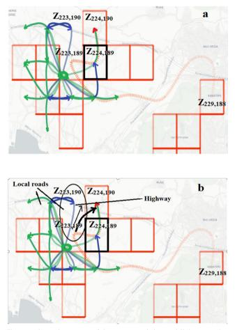
**Fig. 12** The major source of OD-ID = 7 and the road linkage starting from  $Z_{223,189}$ . *Note*: in both **a** and **b**, the black grid represents  $Z_{224,189}$ , the red dash curve is the source, and the solid curves in green and blue are the road connections starting from  $Z_{223,189}$ . The black curve, circle, and arrow in **b** refer to the missing link, the area for the mismatch, and the proposed new road, respectively
