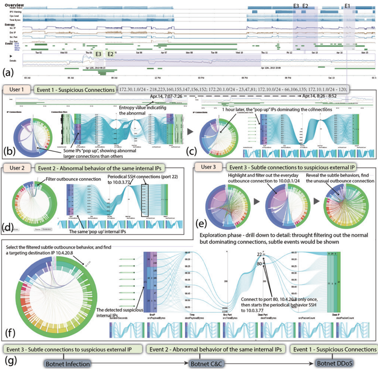
Figure 10: Botnet analysis. (a) Overview timeline. (b,c)-E1, firstly detected events, which turned out to be a botnet DDoS attack. (d)-E2, secondly detected events. By applying filters, user found the suspicious outbound SSH connections. (e,f)-E3, botnet infection as subtle event. (g) Summarized attack pattern.
